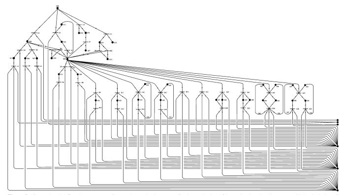
Figure 3. Comprehensive flowsheet corresponding to the maximal structure for the production of butanol, ethanol, and acetone with the inclusion of pervaporation: P-graph representation. A letter followed by a numeral adjacent to a bar designates an operating unit represented by the bar; a letter followed by a numeral adjacent to a small solid circle designates a stream of the material represented by the circle.
