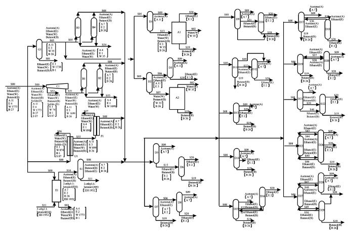
Figure 2. Comprehensive flowsheet corresponding to the maximal structure for the production of butanol, ethanol, and acetone with the inclusion of pervaporation: conventional representation with the component flow rate in  $10^3$  lb/h.
